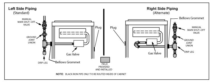
Figure 61. Gas Piping Upflow Applications
