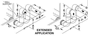
\* Use wall support every 24" (610 mm). Use two wall supports if extension is greater than 24" (610 mm) but less than 48" (1219 mm).
