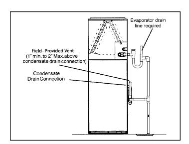
Figure 57. Evaporator Coil Using a Common Drain
