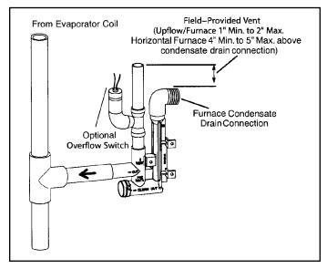
Figure 54. Condensate Trap with Optional Overflow Switch
