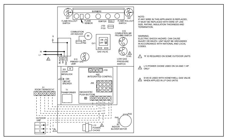
Figure 66. Typical Field Wiring Diagram
