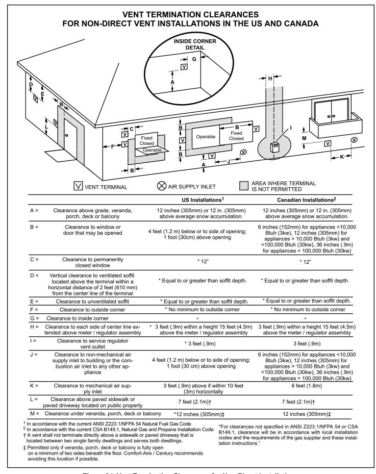
Figure 34. Vent Termination Clearances for Non-Direct Installations
