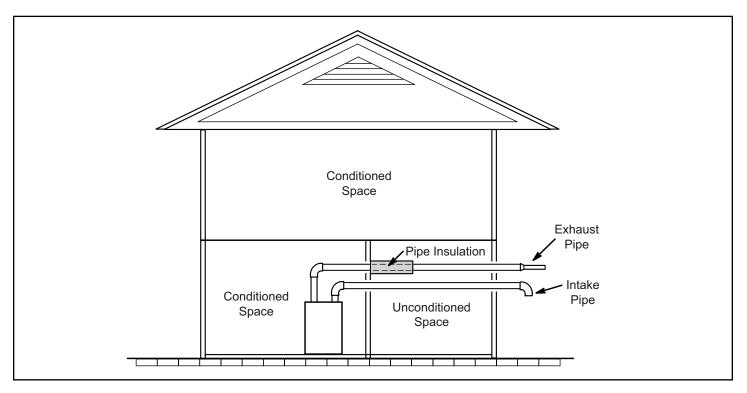
Figure 33. Insulating Exhaust Pipe in an Unconditioned Space
