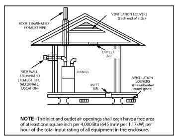
Figure 6. Equipment in Confined Space - All Air from
