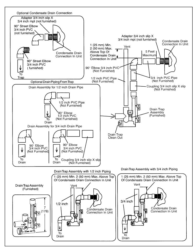
Figure 59. Trap / Drain Assembly Using 1/2" PVC or 3/4" PVC
