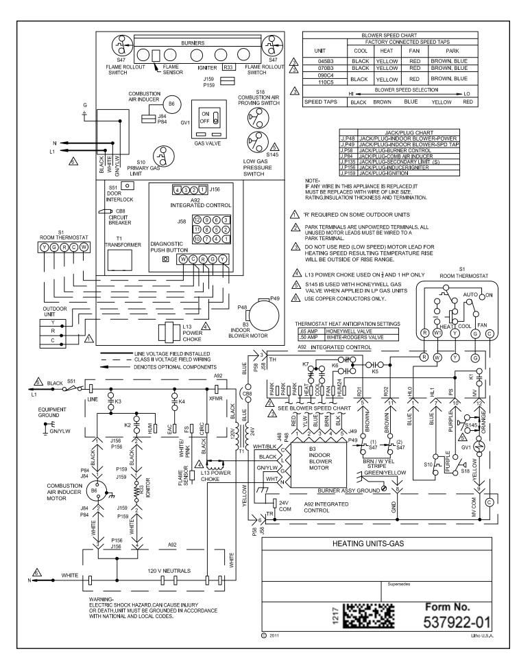
Figure 67. Typical Wiring Diagram
