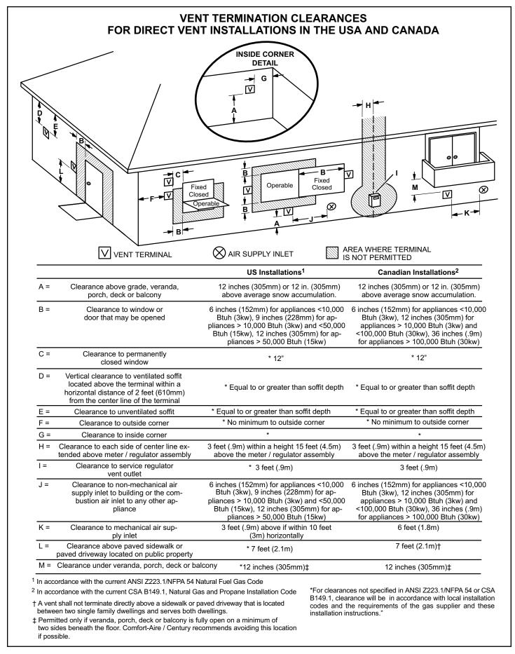
Figure 35. Vent Termination Clearances for Direct Installations
