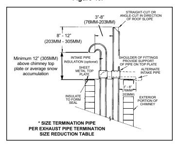
Figure 44. Direct Vent Application Using Existing Chimney
