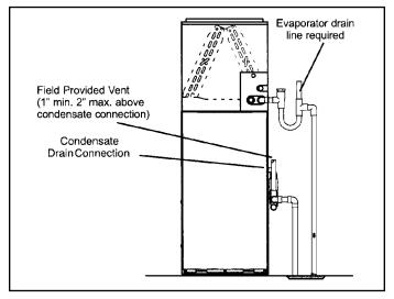
Figure 56. Unit with Cooling Coil Using Separate Drain
