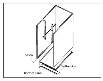
Figure 16. Removing the Bottom Panel
