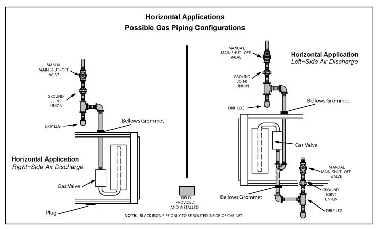
Figure 62. Gas Piping Horizontal Applications
