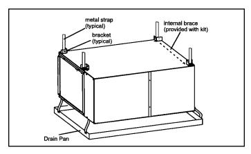
Figure 19. Typical Horizontal Application
