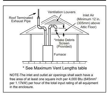
Figure 31. Equipment in Confined Space (Inlet Air from Ventilated Attic and Outlet Air to Outside)
