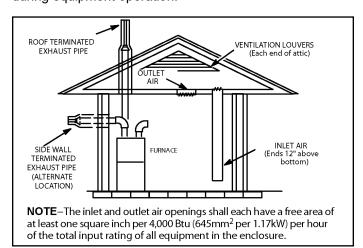
Figure 7. Equipment in Confined Space - All Air from
