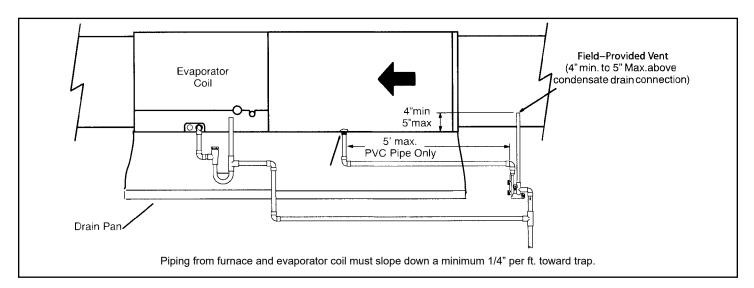
Figure 58. Evaporator Coil Using a Common Drain
