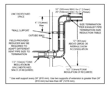
Figure 47. Non-Direct Vent Field Supplied Wall Termination Extended
